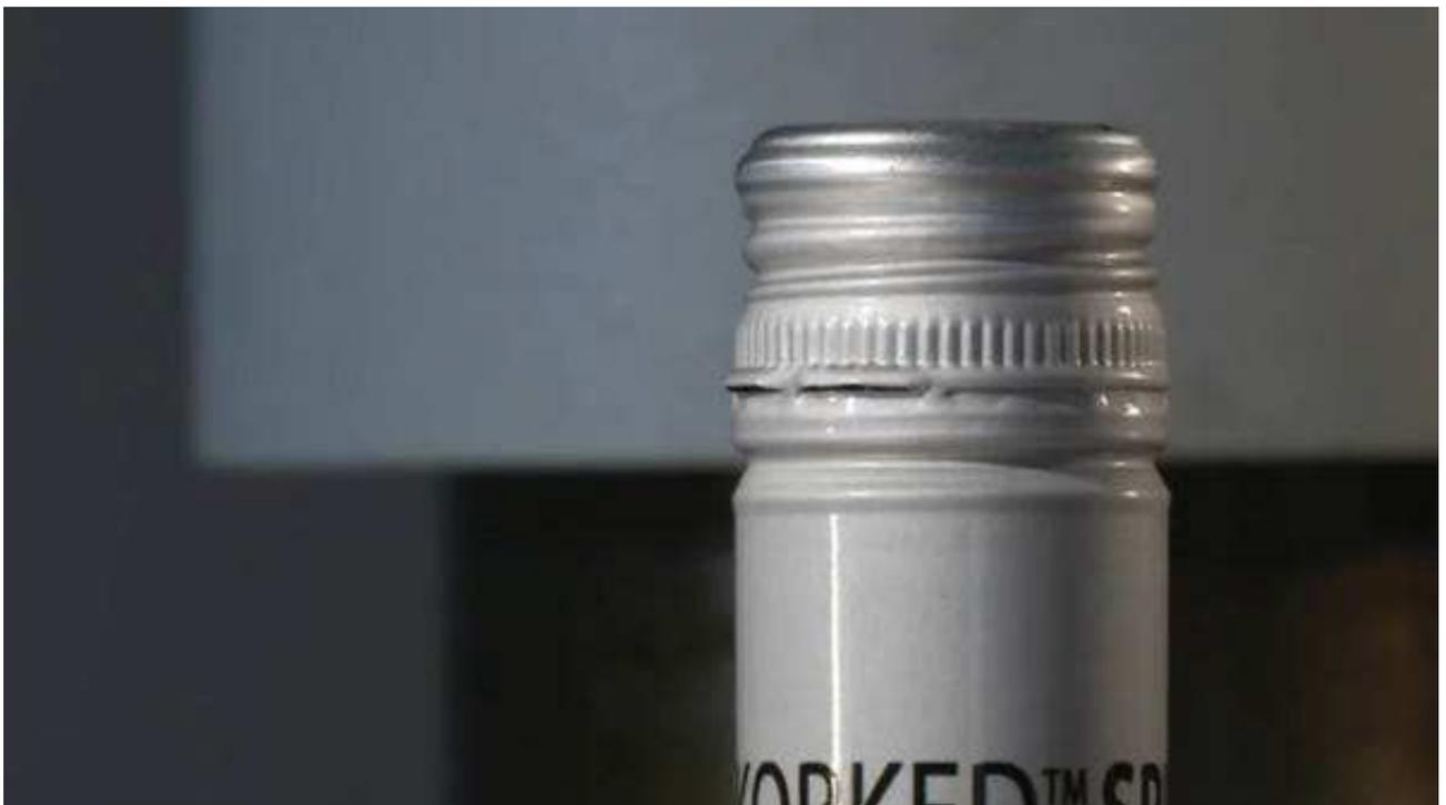
The aluminium between screw cap's bridges tends to deform or flanging in consequence of the following causes:
